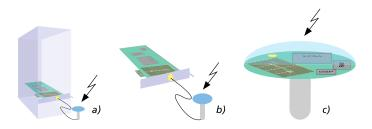
Complete, end-to-end development chain platform: a) hardware platform with PC software; b) software integrated in the receiver hardware c) hardware and software with combined "smart antenna" © Fraunhofer IIS | Images available in color and print quality: www.iis.fraunhofer.de/en/pr.
